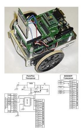
When the BOT receives one of the turning, stop, or backup commands, the BOT executes the movement and then stops and asks for the next command. If no command is forthcoming, the BOT continues to wait. If the BOT is moving forward, it will move forward for approximately 10 inches, stop, send a prompt to the Palm, and if no command is received, the BOT will continue forward an additional increment. If an alternative command is received, that command is executed and the BOT waits.
