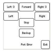
Basically the Palm software displays directional keys on the screen and opens the serial port of the Palm to the SureLink transceiver. When the user touches one of the control buttons, a command represented by a letter is placed in a transmission cue awaiting a signal from the BOE/BOT that it is ready to receive the command. Once the go-ahead is received, the Palm sends the command to the SureLink for transmission.
