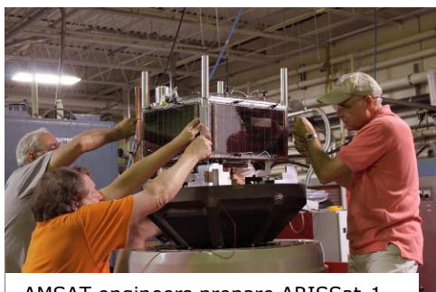
AMSAT engineers prepare ARISSat-1 for vibration testing.
