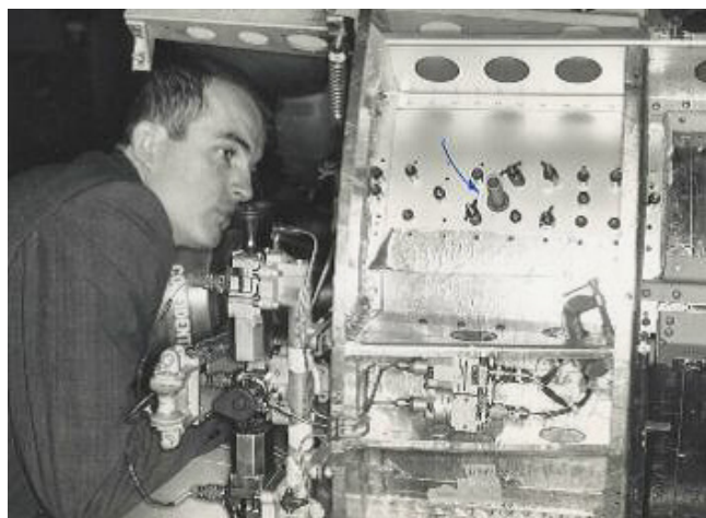
Figure 3 — K6GSJ working on the upper stage of the Thor-Agena A rocket. The transport capacity for OSCAR-1 and ejection mechanism can be seen. Note the curved shape to conform to the exterior surface of the carrier rocket.
